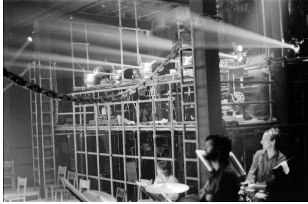
Fig 9: Brunel (Downie, et al., 1981): six electronically linked 16mm projectors with a single roll of film beginning on the far side and taking up on the near side (at right of picture).
